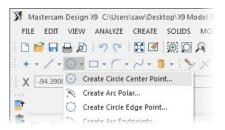
**5** Draw a circle centered on the part, with a diameter (100mm) that matches the outmost circular edge of the part.
