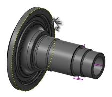
4 Change the chamfer's distance to 5mm
