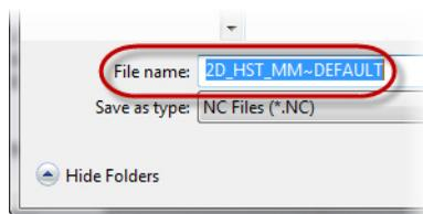
Mastercam for SOLIDWORKS analyzes all operations and creates the NC file for the part. Because you selected the **Edit** option, the NC file displays in Mastercam Code Expert Editor, as shown in the following picture.
