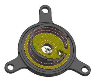
9 In the function panel, make sure that Wireframe is selected, and Project using construction plane is deselected. Then click OK.
