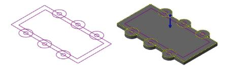
**4** Extrude the inner rectangle upward by 10mm. (For help, refer to page 12.)
