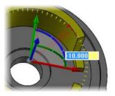
The gnomon's X axis rotates to center on the opening in the vertical wall, as shown (in top view).
