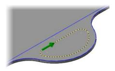
Mastercam adds the chain to the extrude operation, cutting the handle opening.
