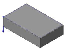
**7** Set the extrude **Distance** to **2**, and press [**Tab**] to accept the new setting.
