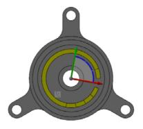
6 Click the gnomon's button to change back to geometry manipulation mode, and ensure that the **Snap to AutoCursor positions** option is selected in the function panel.
