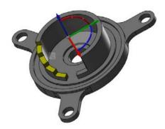
**4** Switch back to geometry manipulation mode, and rotate the geometry -12.5 degrees.
