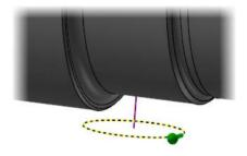
4 Chain the line indicated in the picture to the right. This line is the sweep's along curve.
