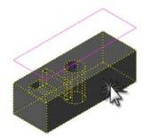
7 Delete the original solid body and rotate the new one to see the solid impression.
