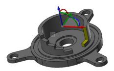
8 Switch back to geometry manipulation mode, rotate the selected geometry 12.5 degrees, and click **OK** in the function panel.
