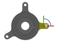
**11** Switch to gnomon manipulation mode, and move the gnomon to the center of the part.
