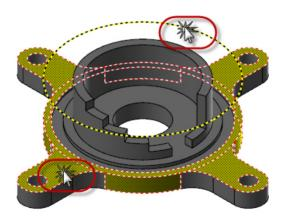
9 In the Split Solid Face function panel, make sure Wireframe is selected and Project using construction plane is not selected.
