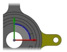
**12** Switch back to geometry manipulation mode, and rotate the gnomon 30 degrees clockwise (-30 degrees).
