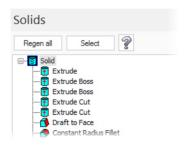
Mastercam's Model Prep functions let you modify solid models lacking a history tree. Mastercam can identify individual geometry elements and even entire features. Using Model Prep functions such as Push/Pull, Move, and Split Solid Faces, you can make changes to a solid, despite having no access to the model's original wireframe.
