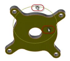
13 In the Split Solid Face function panel, ensure Wireframe and Project using construction plane are selected.
