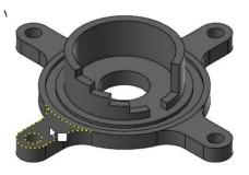
This is the foot you will remove from the part. Mastercam highlights the foot and places a red single-axis arrow control on its face.
