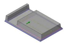
Mastercam extrudes the two chained rectangles, as shown in the picture to the right.
