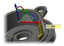
By rotating each side of the opening by 12.5 degrees, you added 25 degrees to the opening, while maintaining its centering on the foot's hole. Your part should now look like the picture below.
