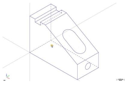
It appears that you have picked up the part and are moving it in the direction of the mouse. However, the entities are not physically moved in space, only the display changes. The Gview does not change as you pan the entities.
