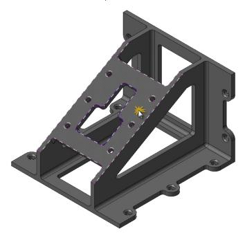
**3** In the Select plane dialog box, click the arrows to cycle through the possible views. For most applications, it make sense to have +Z pointing away from the part.
