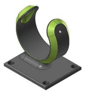
The toolpaths included in the part file machine the green area of the part. This part is ideal for 5-axis toolpaths, because you can potentially machine the whole part in one setup. This would be difficult on a 3-axis machine.
