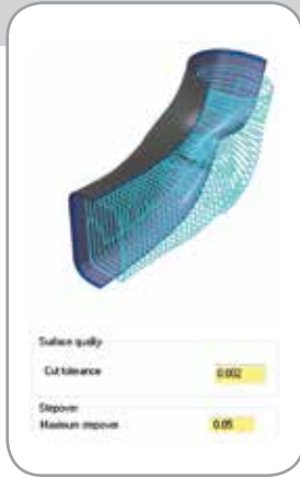
Select the port surface(s) and cut pattern
