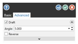
Mastercam updates the display to show the draft on the extrusion. If you have difficulty seeing the draft on the part, toggle the Draft option several times, watching how the part's geometry changes.
