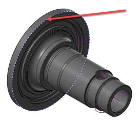
4. Change the chamfer's distance to 5.
