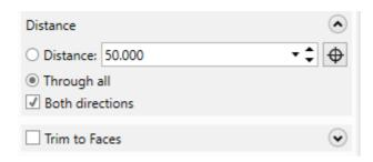
Mastercam cuts the shape specified by the chained geometry through both sides of the boss, giving the results shown.
