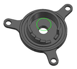
If the circle is laying completely on top of the solid, you would have to turn off the face filter in general selection to pick the circle. When the circle is positioned over empty space it can be selected without changing the filter.
