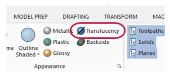
The part becomes partially transparent, allowing you to see the two new rectangles hidden under existing geometry.
