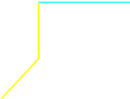
13. Draw a line from the previous line's endpoint, giving it a **Length** of 25 and an **Angle** of 270.
