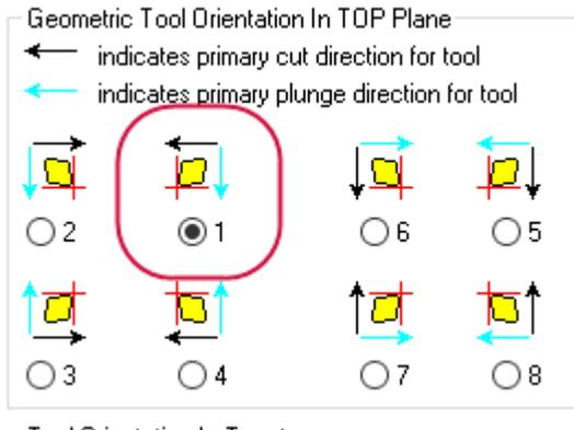
This is the orientation of the tool's geometry as it is viewed in the Top plane. Note that choices 1 and 5 have the same geometric orientation, but the cut and plunge directions are different. Orientation 5 is typically used for horizontal tools.
