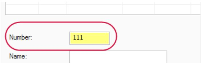
Because tool geometry must be on its own level, with no other geometry, you should pick a level number that you are unlikely to use in your part drawings.
