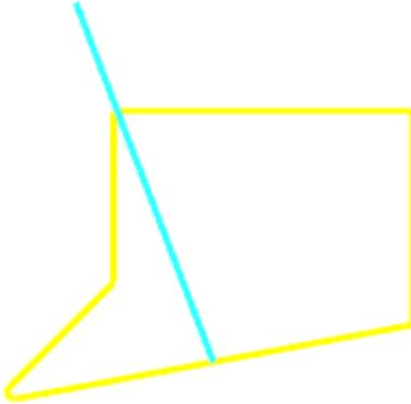
4. Draw a line from the top end of the previous line, setting its **Length** to **210** and its **Angle** to **90**.
