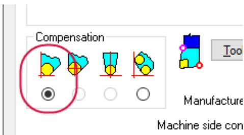
This selection specifies that compensation for a toolpath is based on the sharp corner of the tip corner radius.
