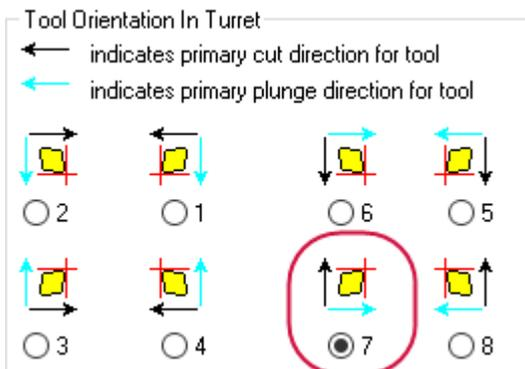
This is the orientation of the tool as it will be mounted in the turret. Note that, again, choices 3 and 7 have the same geometric orientation, but the cut and plunge directions are different.
