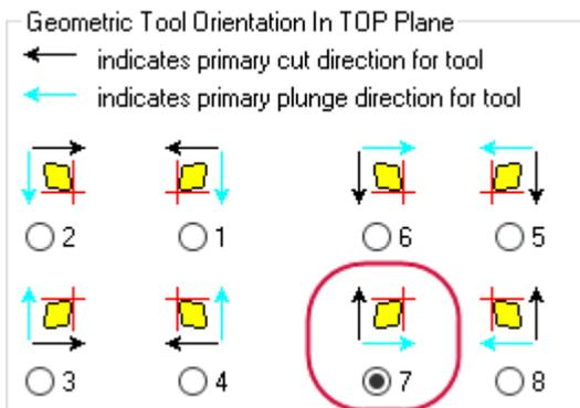
This is the orientation of the tool's geometry as it is viewed in the Top plane. Note that choices 3 and 7 have the same geometric orientation, but the cut and plunge directions are different.
