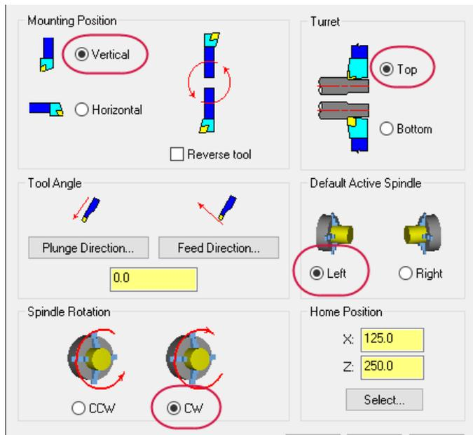
Your settings (except possibly **Home Position**) should match the above image. Notice that, in Mounting Position, the vertical tool picture is oriented as you expect for the upper turret, left spindle.
