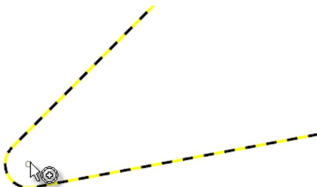
The insert moves to the origin, with the tip arc's centerpoint centered at 0,0.
