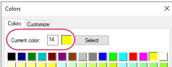
You must use different colors to draw the tool's insert and holder. The recommended color for "insert up" is 14. For "insert down," the recommended color is 138. For the holder, use color 116.
