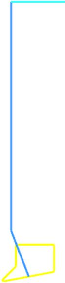
6. Draw a line from the right end of the previous line, setting its length to **247** and its angle to **270**.
