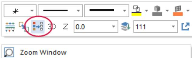
Mastercam restores the geometry to its original colors.
