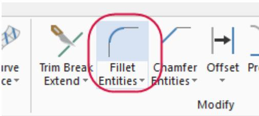
3. Select the tip's two lines, set **Radius** to **0.8**, and click the function panel's **OK** button.
