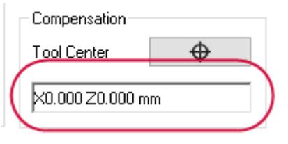
The more common position for a vertically oriented tool is with the insert's driving point fully in the upper-right quadrant of the graphics window. In this case, you would set the compensation point and tool center as shown in the following image.
