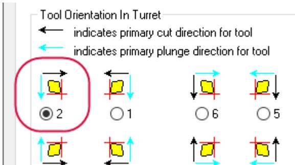
**Note:** Make sure that you change the **Tool Orientation In Turret** setting and not the **Geometric Tool Orientation In TOP Plane** setting. Because the geometric orientation is based on how you drew the tool in the graphics window, you do not need to change it once it is set.
