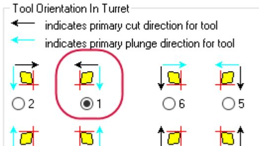
This is the orientation of the tool as it will be mounted in the turret. Note that, again, choices 1 and 5 have the same geometric orientation, but the cut and plunge directions are different.
