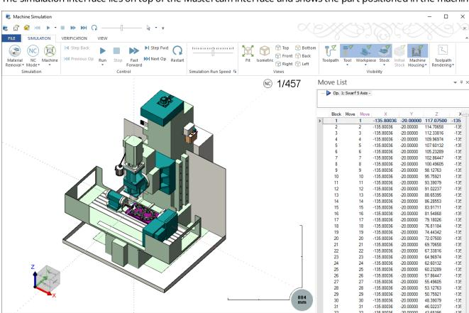
The simulation interface lies on top of the Mastercam interface and shows the part positioned in the machine.
