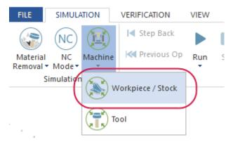
This focus option moves the tool around a stationary workpiece.
