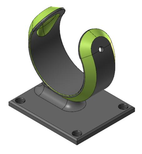
The toolpaths included in the part file machine the green faces on the part. This part is ideal for 5-axis toolpaths, because you can potentially machine the whole part in one setup. This would be difficult on a 3-axis machine.
