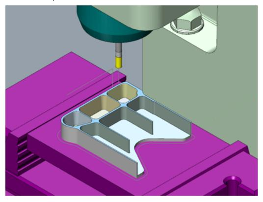
11. When the simulation is complete, click **Exit** to return to the main Mastercam screen.
