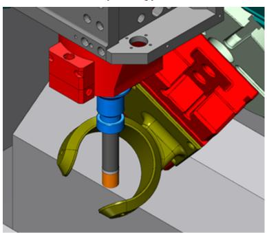
The fixture is colliding with a section of the tool spindle.
