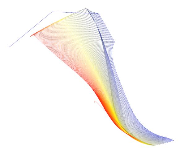
The default colorization uses ten gradients, starting with red at the beginning of the toolpath and ending with blue. You can see where the toolpath begins and ends and that it moves in a zigzag pattern.
