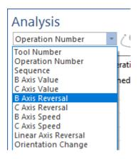
This analysis option changes the toolpath color every time the rotation axis changes direction. The color changes can help you identify areas where direction changes could impact your surface quality.
