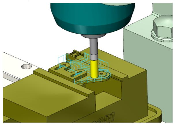
10. When the simulation is complete, click **Exit** to return to the main Mastercam screen.
