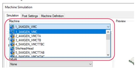
Mastercam includes models of the most popular mill and router machines in the industry, including examples of all three major 5-axis machine groups.
