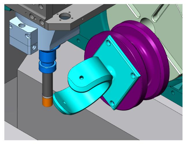
You can see the tool actually removing material from the part as it moves through the toolpaths.
