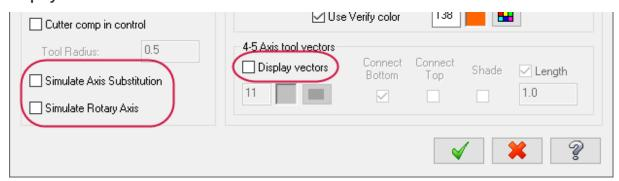
Turning these options off keeps the part stationary in the graphics window and moves the tool around the part.
