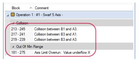
6. Click on **Collision between B1 and A3** in the **Report** tab and Machine Simulation jumps to where the problem occurs. The two axes that collide display in red.
