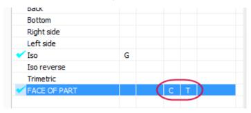
Due to the **Tplane follows Cplane** rule, Mastercam sets both the Cplane and Tplane to the FACE OF PART plane, which contains the slanted slot.
